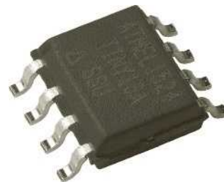
FIGURE 1.1 Microprocessors: (a) General-purpose Intel Core™ i7 CPU; (b) Dedicated Atmel ATtiny13A microcontroller.
