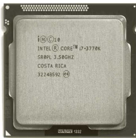
FIGURE 1.1 Microprocessors: (a) General-purpose Intel Core™ i7 CPU; (b) Dedicated Atmel ATtiny13A microcontroller.
