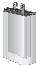
Figure 1-8 Chemical cell as a voltage source. (a) Voltage output is the potential difference between the two terminals. (b) Schematic symbol of any DC voltage source with constant polarity. Longer line indicates positive side.
