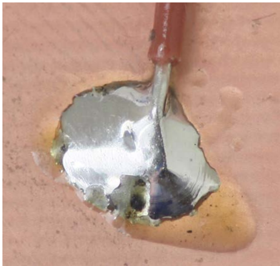
FIGURE 1-3 A good connection where the solder has been heated sufficiently to flow properly.
