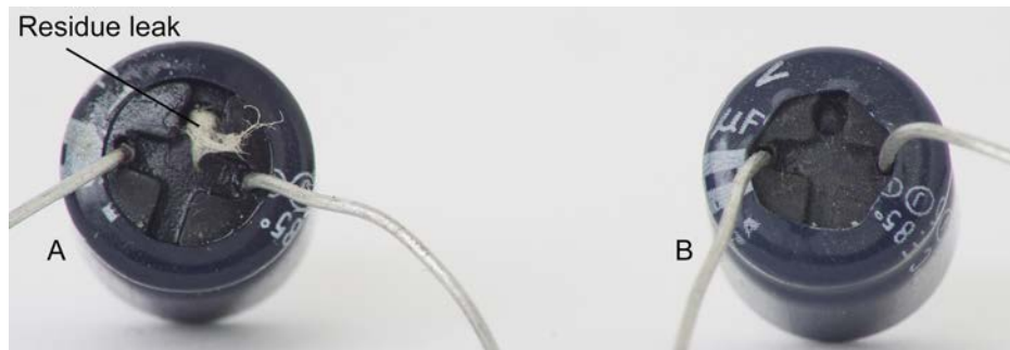
FIGURE 1-1 A bad capacitor on the left side (A), and a good capacitor on the right side (B).
