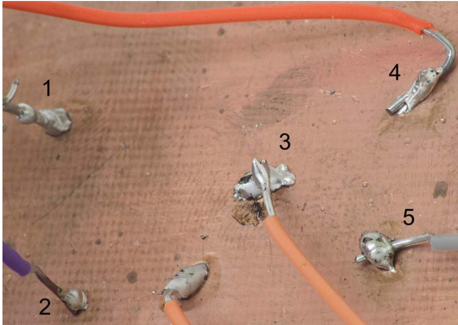
FIGURE 1-2 Bad solder connection examples.
